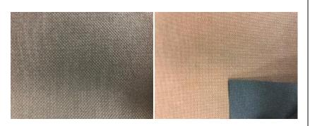
Weed Barrier Pro (or 12 Year Weed Barrier) is a pointbond polypropylene fabric used in professional landscape applications. The fabric is designed to allow air, water, and nutrients to pass through.
